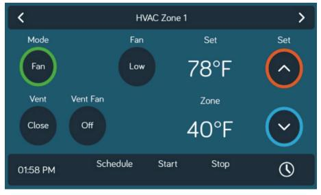
Use the "Set" temperature up and down arrows to set the desired temperature. The "Set" temperature can be adjusted between 55 to 90F.
